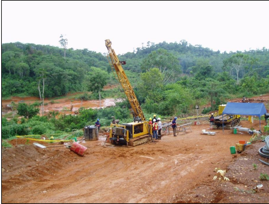
Figure 16 Coretech track mounted diamond drill rig utilized by Reflex Drilling Limited.
