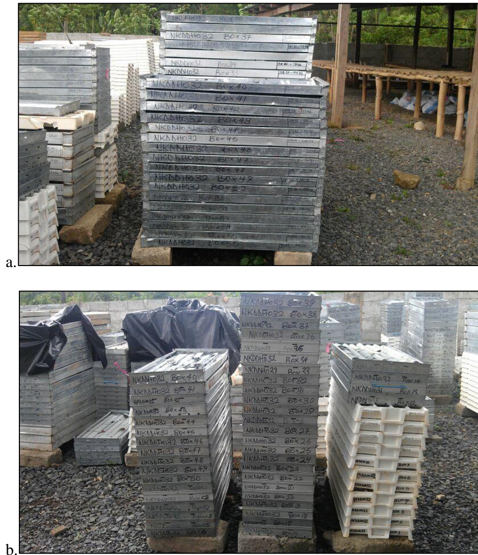
Figure 18 Core storage in both labelled galvanised and plastic core trays at core yard at Kedadwen.
