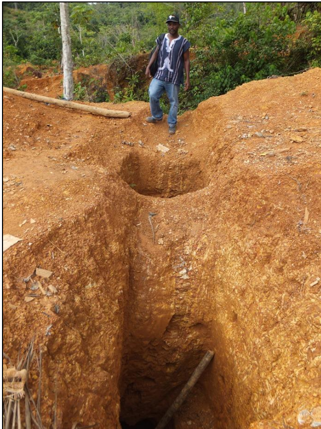
Figure 8 The Apankrah Cross-vein, worked by galamsey ‘shafts’ strikes approximately E-W. Note the vertical dip becoming steep to the S with depth. Main Apankrah trend behind field geologist.
