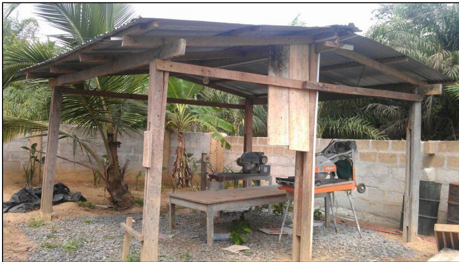
Figure 20 Core saw for sawing core into half longitudinally.
